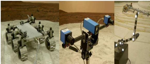
Figure 7: Rover chassis, panoramic and zoom camera with pan/tilt mechanism and manipulator. Images courtesy of UWA.
