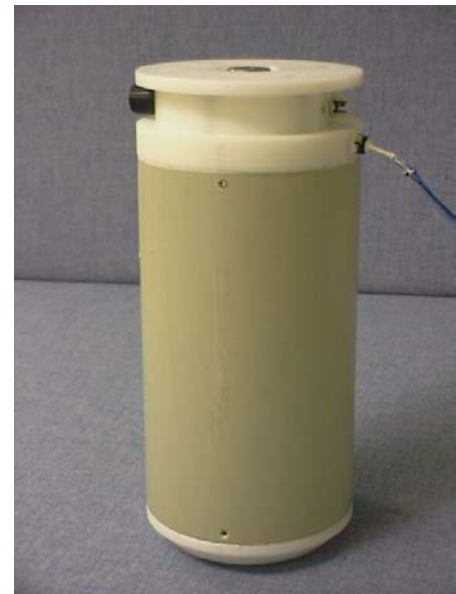
Figure 3. DIVEBOT. (Length: 38 cm, Diameter: 16.8 cm, Weight: 8.4 Kg).
